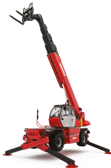
Rotation on lowered stabilizers with 1500 kg jib
